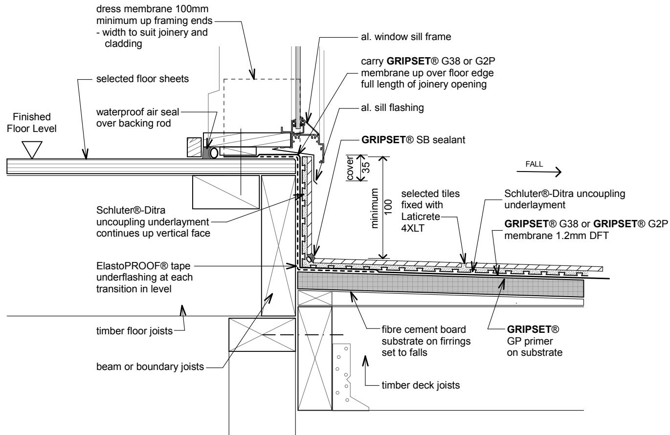
gsM-D03 - Window Sill/ Tiles (on Uncoupling underlayment)-junction - type 1
