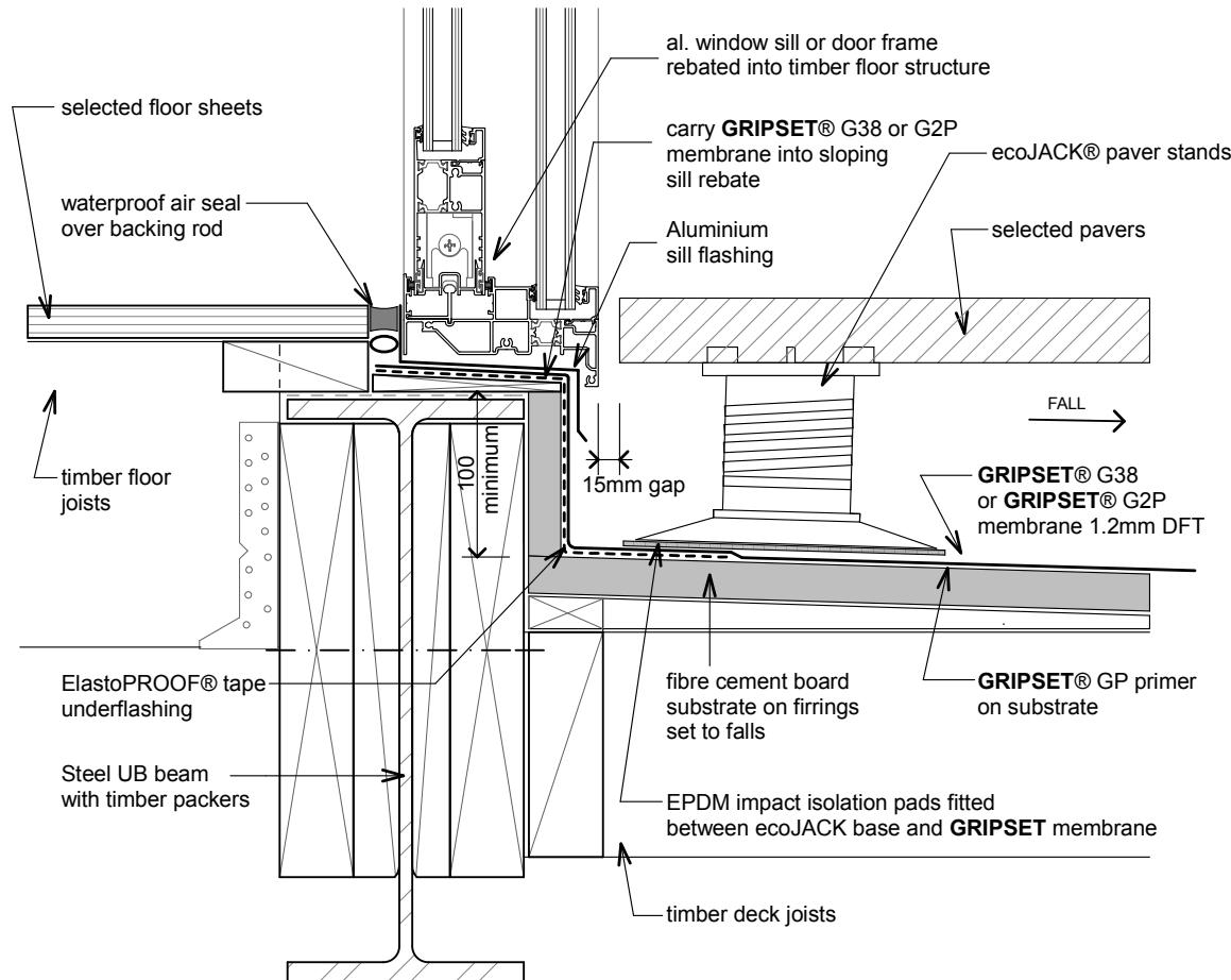
gsM-D22 - ecoJACK® paver-threshold detail - type 2
