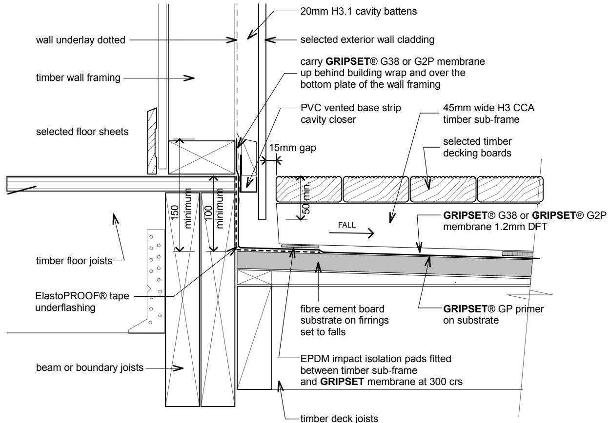
gsM-D25 - timber raft floating deck-wall detail - type 1
