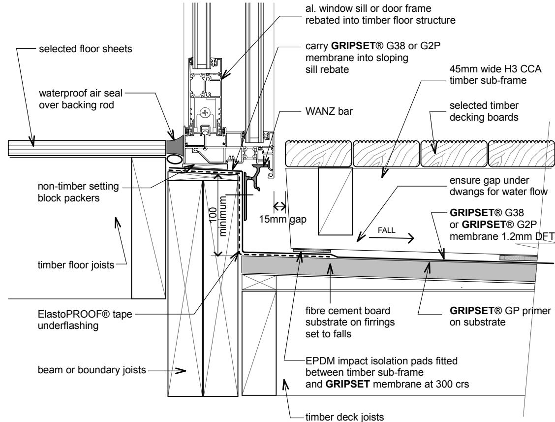
**gsM-D27 - timber raft floating deck-threshold detail - type 1**
