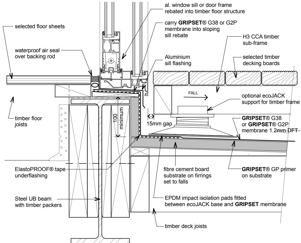
gsM-D28 - timber raft floating deck-threshold detail - type 2
