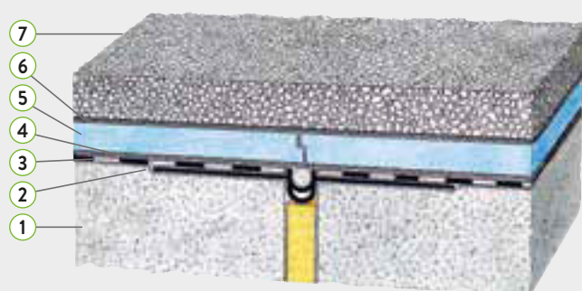
1 Deck 2 Elastic joint 3 PVC-P Membrane 4 Non-woven fabric 5 Insulation 6 Non-woven geo-textile 7 Gravel
