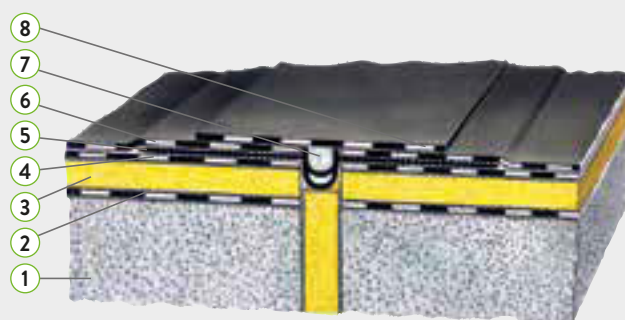
1 Deck 2 Vapour barrier 3 Insulation 4 Membrane 5 Elastic joint 6 Membrane 7 Polyurethane foam filler 8 Partially attached membrane
