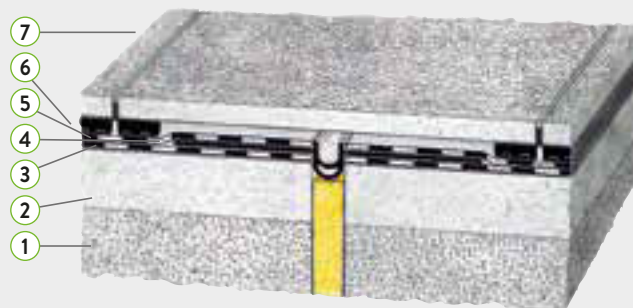
1 Deck 2 Lightweight concrete 3 Membrane 4 Elastic joint 5 Membrane 6 SEALCO LTD supports 7 Paving tiles
