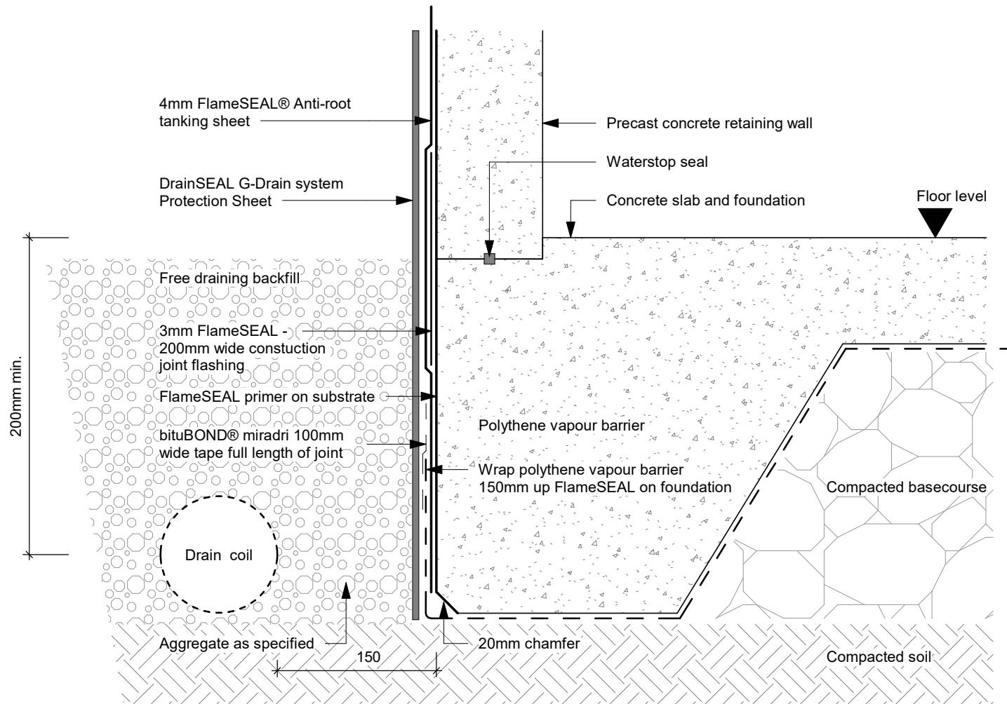
**fS-T D19 - Precast Wall/ Floor Joint (Single Layer)**
