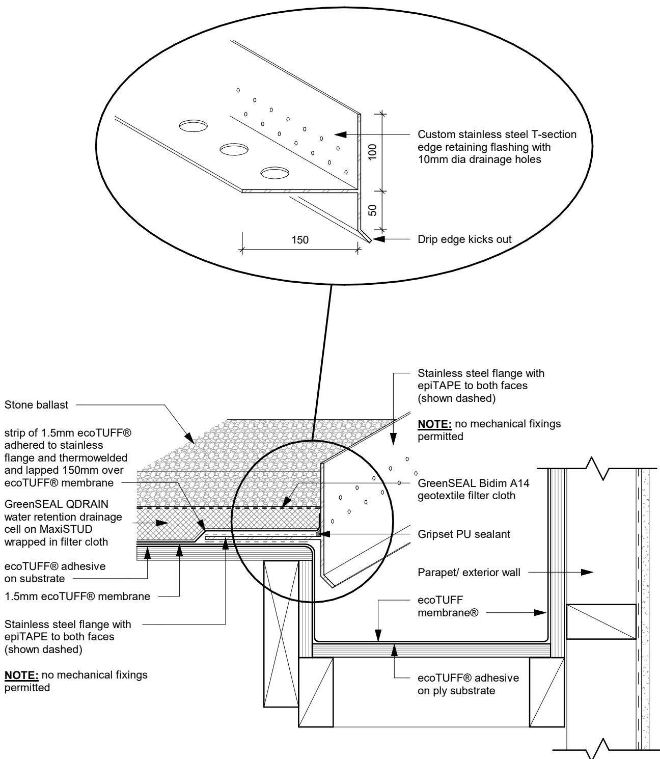
eT D04 (TPO) - Ballast Gutter
