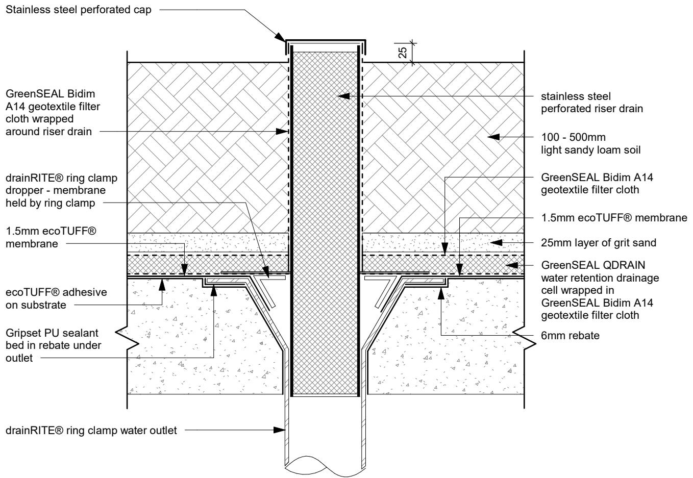
**eT D07 (TPO) - Soil drainRITE® Outlet**
