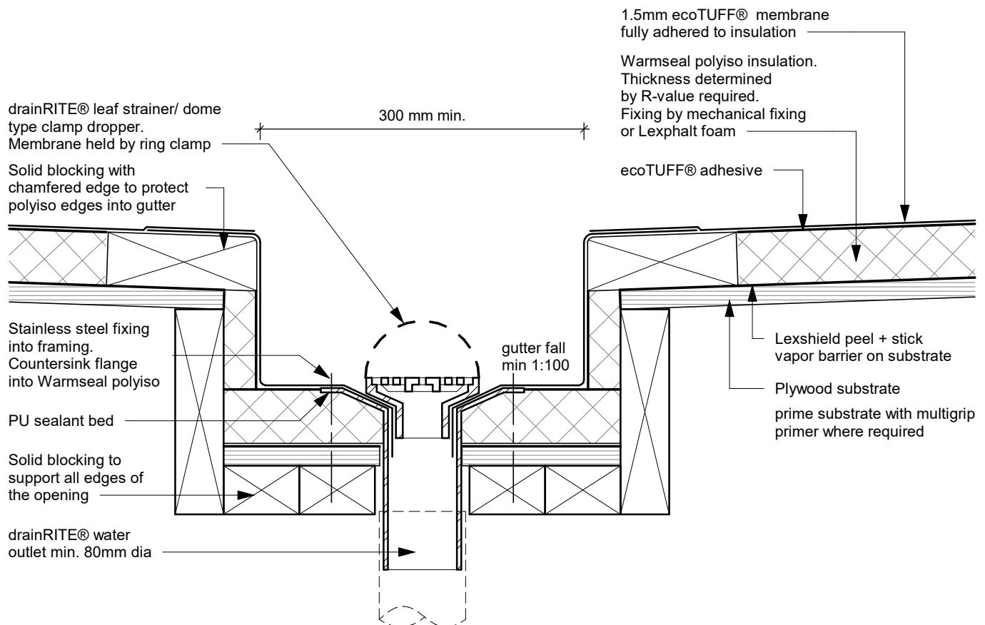
WS ET021 - drainRITE® Water Outlet 5 (Dropper) - Ring Clamped Dome
