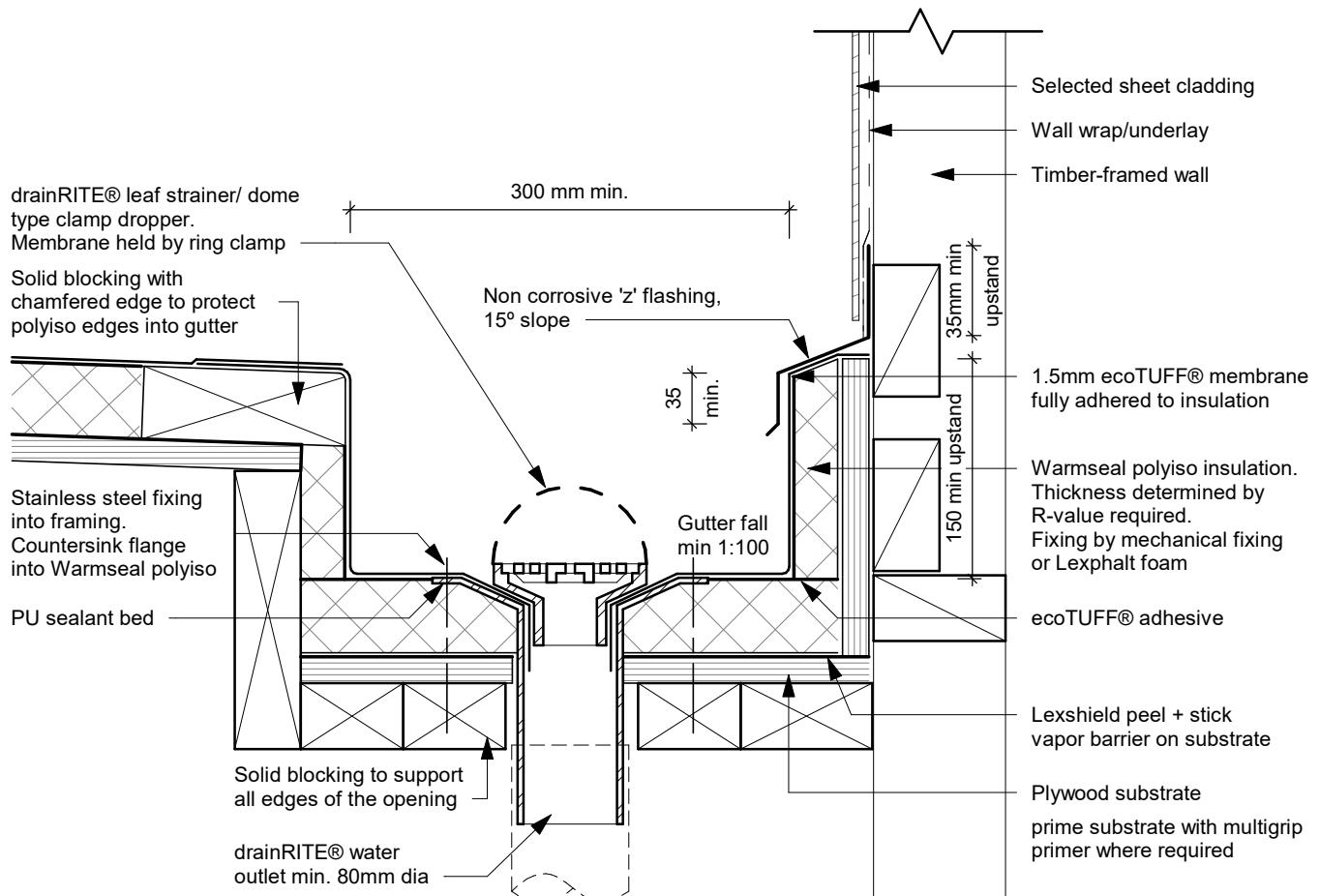
WS ET022 - drainRITE® Water Outlet 6 (Dropper) - Ring Clamped Dome
