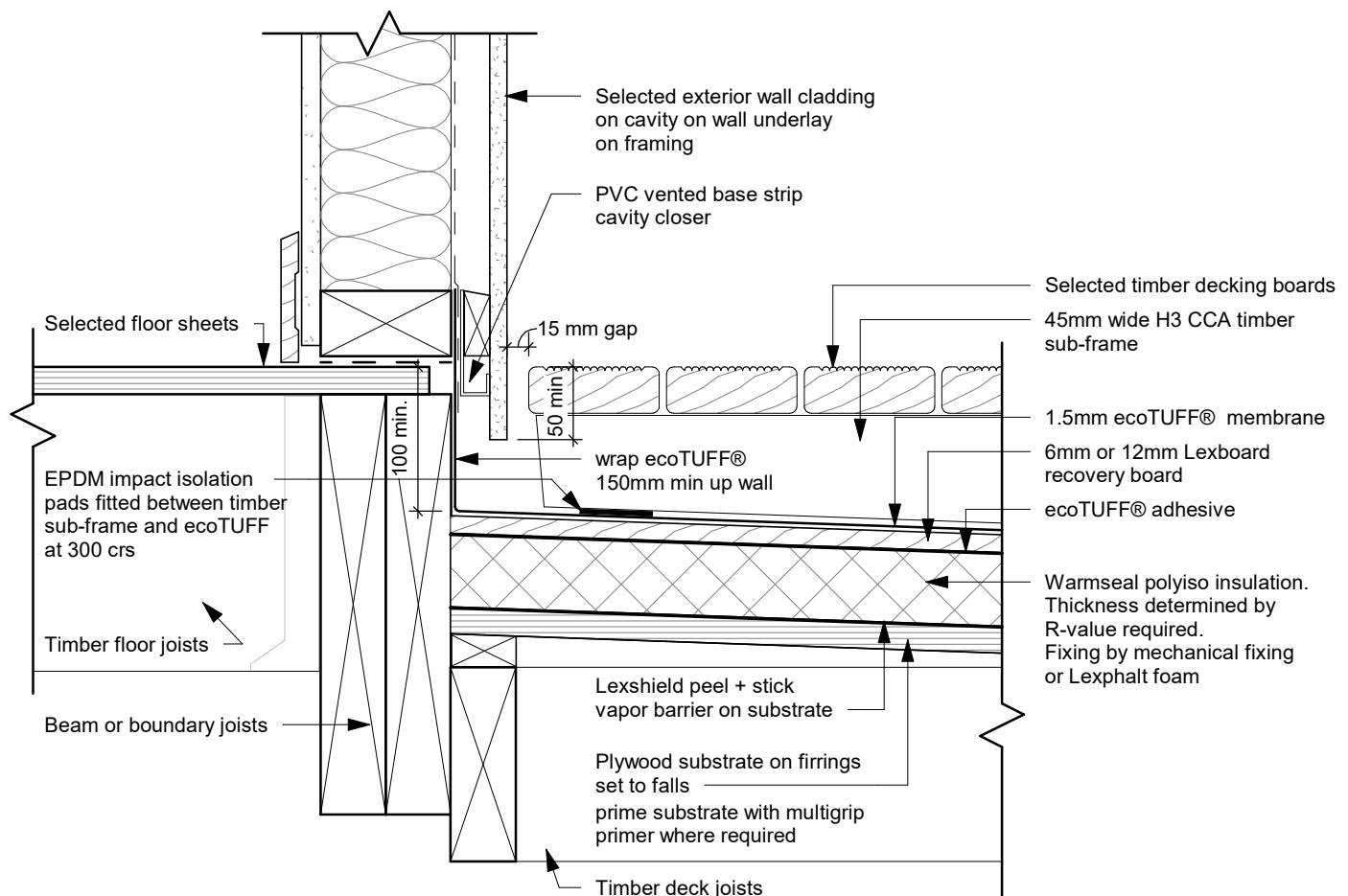
WS ET034 - Timber Raft Floating Deck - Wall Detail - Type 1
