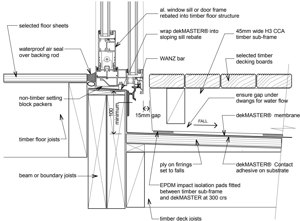
dek-M38 - timber raft floating deck-threshold detail - type 1
